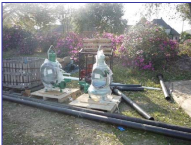
New submersible pumps wrapped from the factory and ready for installation into wet wells.
